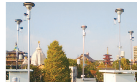
Parallel test of PM2.5 continuous measurement equipments
